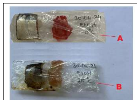
Fig 2. Beetroot based sticker indicating fresh (A) and 24 hours old (B) sardine stored at 0°C and 25°C, respectively.
